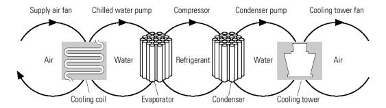
Figure \.\ Heat Transfer Loops In Refrigeration System
