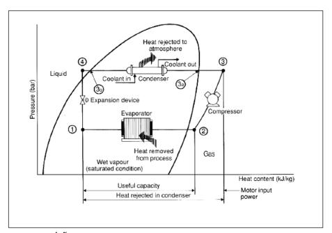
Figure 1. 7: Schematic of a Basic Vapor Compression Refrigeration System
