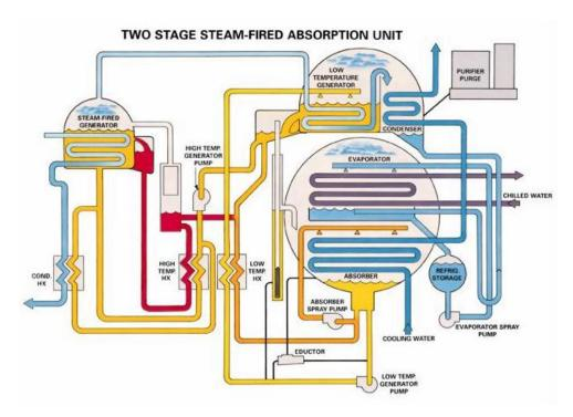
Figure 1. Schematic of Absorption Refrigeration System
